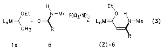
$\text{L}_n\text{M} = \text{Cr}(\text{CO})_5$ ;  $\text{R} = \text{s.Tab.1}$
